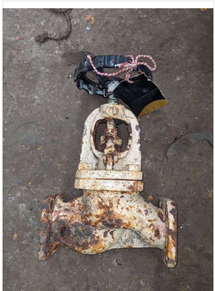
6. Z type globe valve, globe valve, DN- 40
